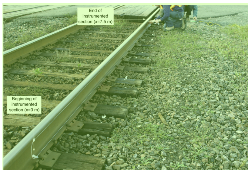
Figure 47. Installation of fiber on rail [120].
